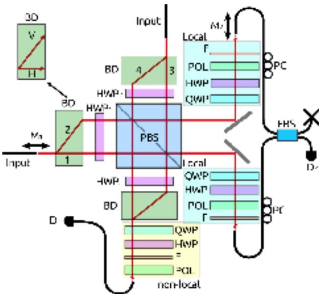
Figure 1: Scheme of the experimental setup. *M* - motorized translation, *HWP* - half-wave plate, *QWP* - quarter-wave plate, *PBS* - polarizing beam splitter, *BD* - beam divider, *POL* - polarizer, *F* - interference filter, *Loc.* - local measurements, *nLoc.* non-local measurements, *D* - detector, *FBS* - fiber beam splitter, *PC* - polarization controller.
